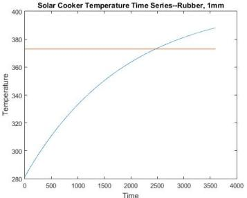
$$\begin{aligned} Q_{cond} &= \frac{kA\Delta T}{d} \\ Q_{rad} &= \pi r_{shell}^2 * \frac{k_i}{m^2} * sin(\theta) \\ \frac{dE_{pot}}{dt} &= Q_{rad} - Q_{cond_{p,a}} \\ \frac{dE_{air}}{dt} &= Q_{cond_{p,a}} - Q_{cond_{a,e}} \end{aligned}$$
