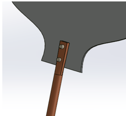
Figure 8: The rivet, used throughout the sculpture, reliably holds together the many sheet-metal parts.
