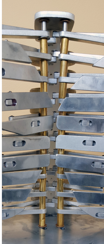
Figure 3: The shaft-support plate on top, along with the main baseplate, are connected by a shaft; all of which, together, create an I structure.
