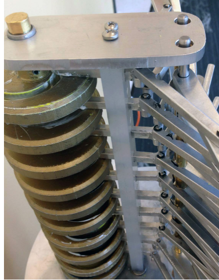
Figure 5: The shaft-support plate and the supporting columns(which house the holes through which cam followers go through) form a T structure.
