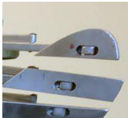
Figure 13: The loctite between the wing skeleton and the image holds the two pieces together.
