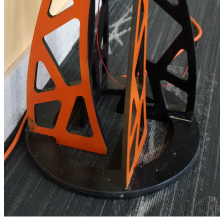
Figure 8: The Legs of the base and the bottom plate of the base are joined by a lap joint, aided by wood glue.
