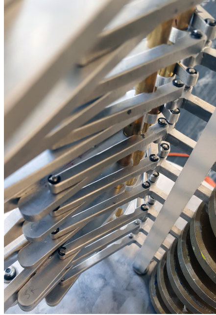
Figure 16: 4-bar linkages actuated by the follower attached to the cams.
