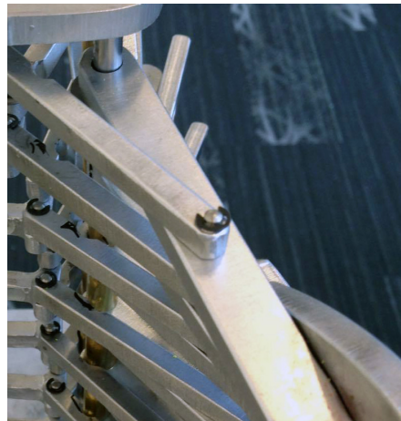
Figure 12: The retaining ring placed on the dowel pins keep the wing supports from falling.
