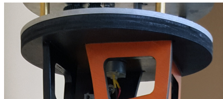
Figure 7: The legs of the base and the top plate of the base are joined by a rabbet joint, with slots on the top plate, aided by wood glue.
