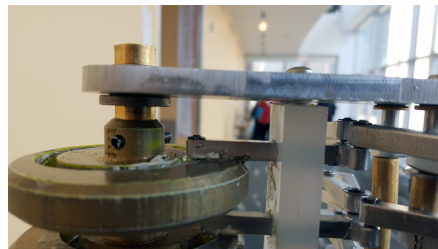
Figure 2: The cam and the supporting columns together form a c structure, on which the cam follower rests.
