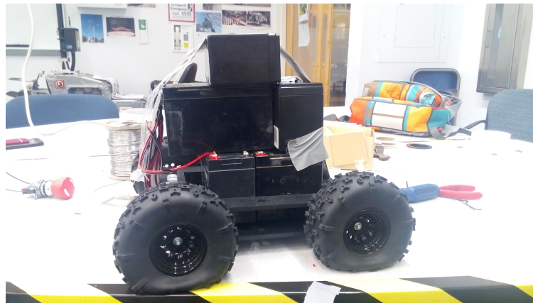
Figure 8: Under the anticipated load of 25 pounds, the wheel was blatantly collapsing, which raised concerns about frictional force and overloading.
